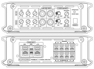
The DB Drive Euphoria 4 channel amplifiers (FX90.4 and FX125.4) feature a 12db Slope crossover network. Channels 1 and 2 can be used in the High pass setting or full range and channels 3 and 4 feature a selectable 3 way crossover system that can be used in High pass, Bandpass or low pass settings.
