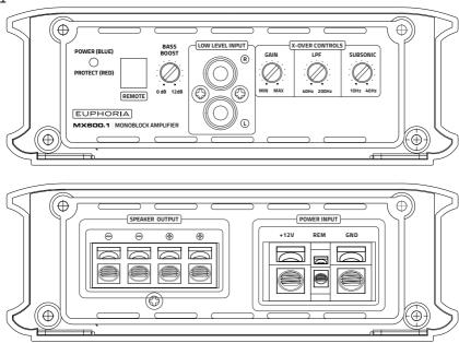
The MX600.1, MX1200.1, MX2000.1 are equipped with a variable 12db slope Lowpass crossover network and a 12db slope subsonic filter. The mono amps also feature a variable Bass Boost EQ is set at 45Hz. The Bass Boost is helpful in certain subwoofer installations where enclosure location may require an extra boost.
